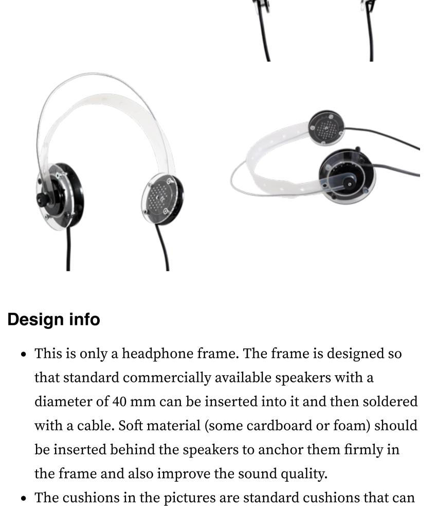
• According to the Ikego catalogue, the outer wire is 2 mm thick. In all of our prototypes, it was so strong that it could be bent, but also had enough strength of its own to exert just the right amount of pressure to press the headphone cups onto the ears. • Assembly outer side:
